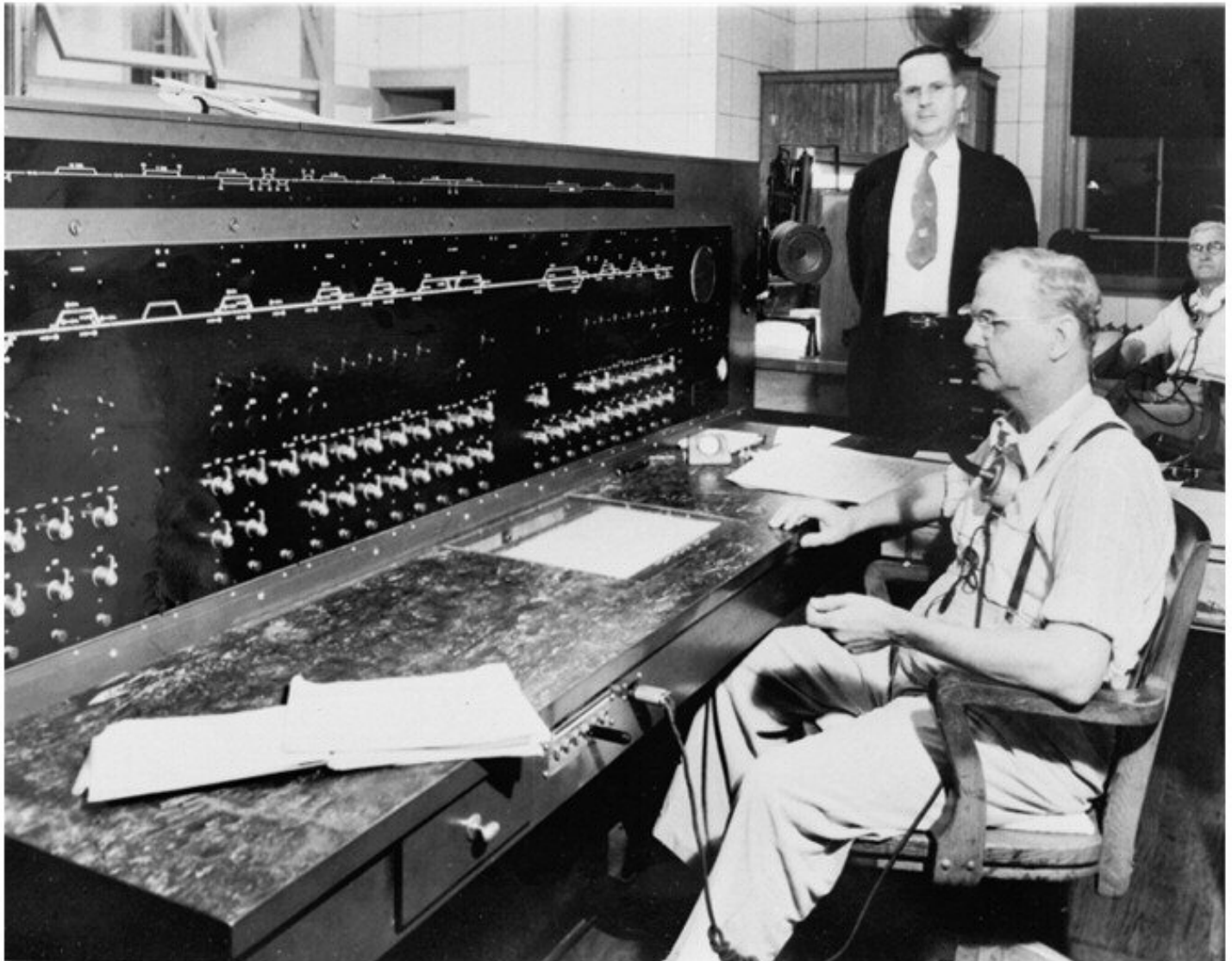
Second trick dispatcher Frank Simmons is sitting at the new GRS CTC console at Mobile in 1943. This machine controlled Flomaton to Sibert on the M&M Sub-Division. Stations on the board include (left to right) Miles, Wawbeek, Canoe, Atmore, Perdido, Dyas, Bay Minette, Hurricane, Nenemoosha, Akka, Aladocks and Three Mile Creek. Device in center of desk is electric graph which automatically keeps up with signalling and track occupancy. Assistant Superintendent B. H. Harbin and fellow dispatcher D. L. Laxton, working the NO&M Sub-Division, look on.
